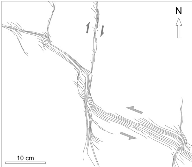
Fig. 5. Line drawing of an early sinistral shear zone cut by sets of late dextral shears. Although it cannot be excluded that some pulses of sinistral shearing succeeded or accompanied dextral shearing, most of the sinistral shearing preceded the dextral shearing.
